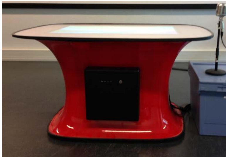
Figure 4: The multitouch table of the HMI research Group using the Rear Diffused Illumination principle.
